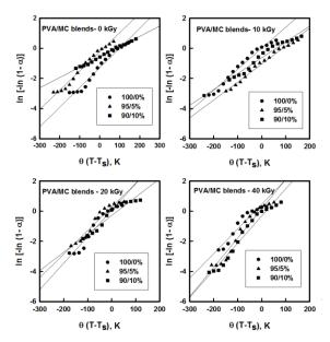
Fig.5. Plots of ln ln  $(W_o)/(W_t)$  vs.  $\theta$  where  $\theta = T - T_s$  for gamma irradiated PVA/MC blends at different doses, according to the Horowitz-Metzger equation.
