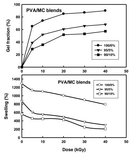
Fig.1. Effect of gamma irradiation dose on the gel fraction (%) and swelling (%) in water at room temperature and pH of 7 of PVA/MC blends of different ratios.
