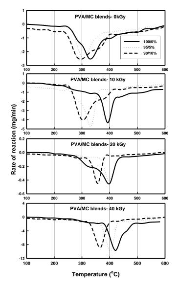
Fig.3. Rate of thermal decomposition curves of PVA/MC blends, before and after gamma irradiation at various doses.
