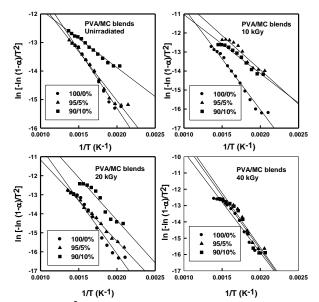
Fig.4. Plots of log  $[g(\alpha)/T^2]$  vs. 1/T for gamma irradiated PVA/MC blends at different doses according to the Coats–Redfern equation.
