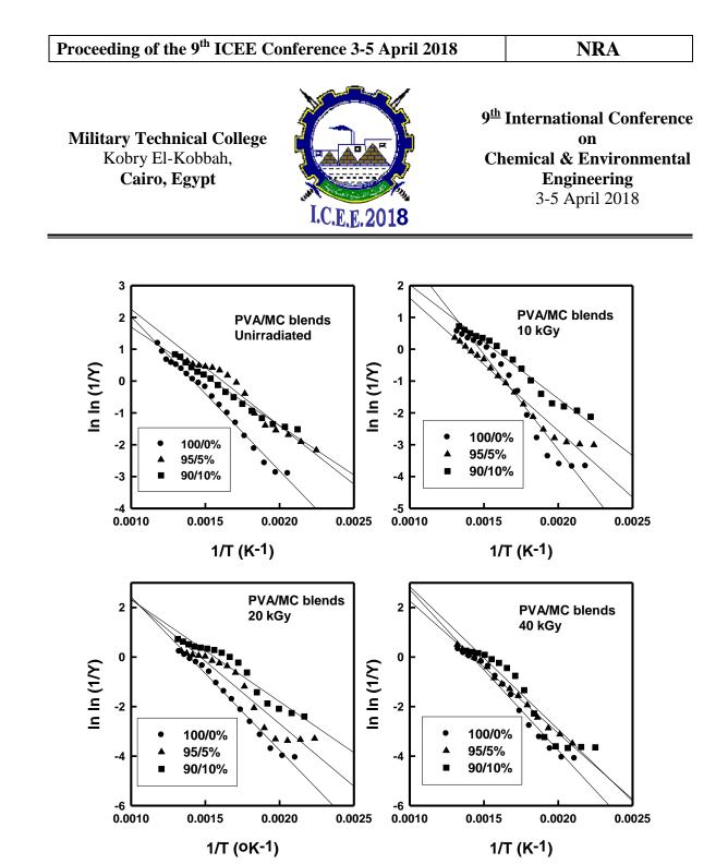
Fig.6. Plots of ln ln (1/Y) vs. 1/T where  $Y = (W_t - W_{\infty})/(W_o - W_{\infty})$  for gamma irradiated PVA/MC blends at different doses according to the Broido equation.
