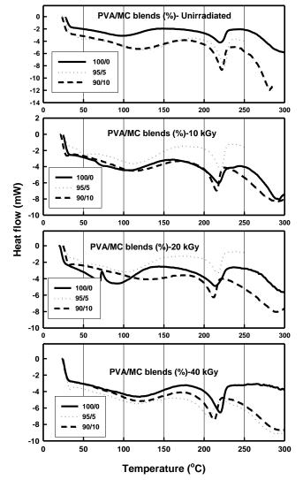
Fig.7. DSC thermograms of gamma irradiated PVA/MC blends at different doses.
