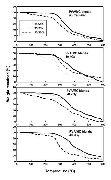
Fig.2. TGA thermogram curves of PVA/MC blends, before and after gamma irradiation at various doses.
