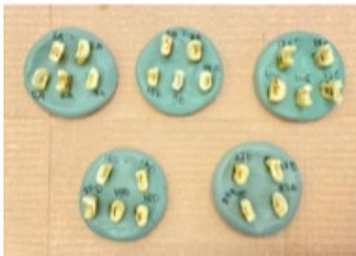
Figure 2: showing photograph of sample arrangement in Silicone mold. All samples are directed toward buccal side with attaching orthodontic wire as a reference.
