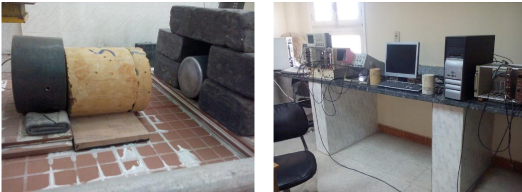
Figure 1: Photo image for fast neutrons attenuation measurements including electronics associated with the stilbene detector.
