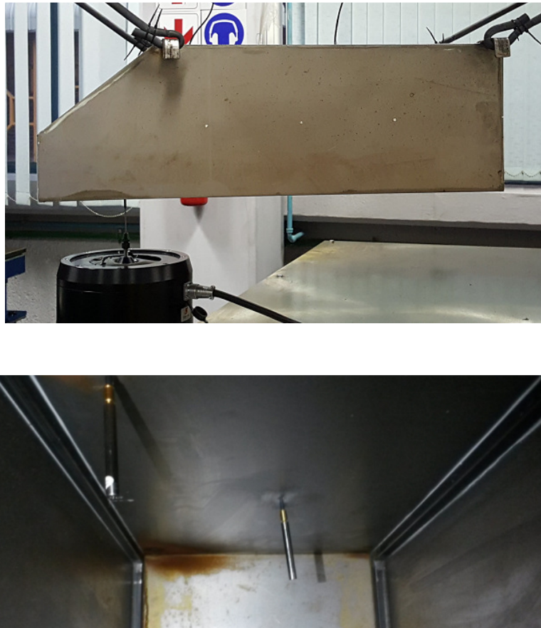
Fig.9. A photograph of constructed cabin with attached microphones.
