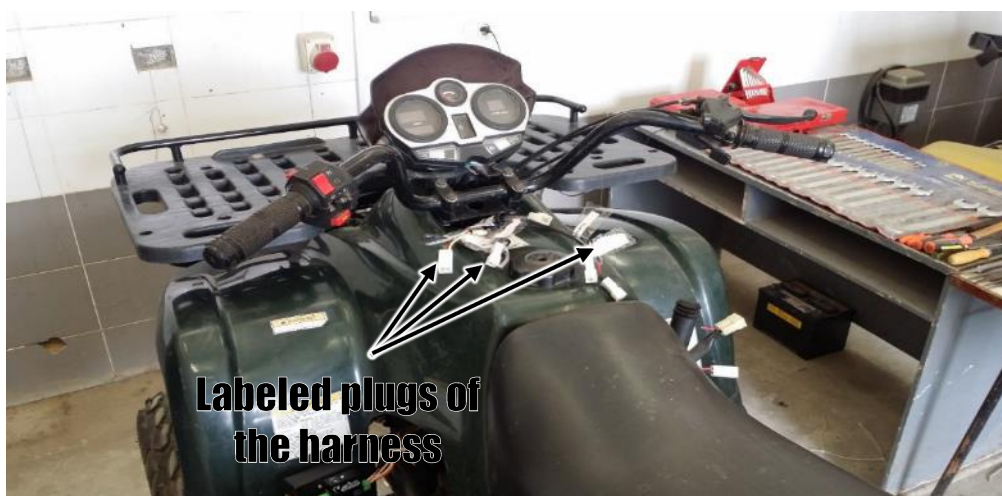
Fig. 14. Labeled plugs of the new harness to facilitate the extended control work.
