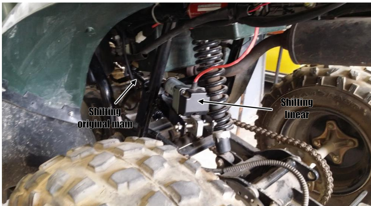
Fig. 10. Shifting linear actuator in its compartment.
