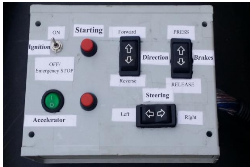
Fig. 13. Wired control panel.
