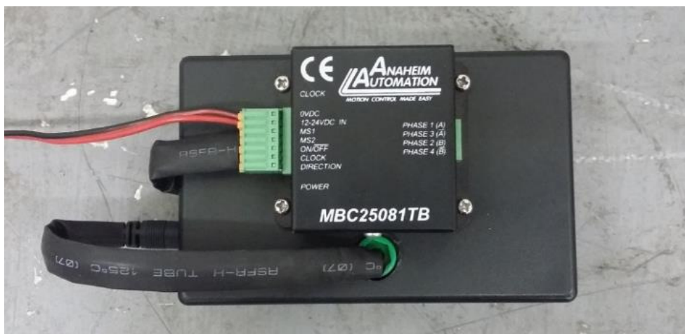
Fig. 8. Controller and driver of the accelerator stepper motor.
