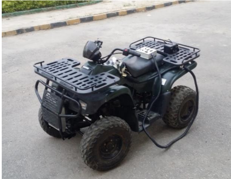
Fig. 16. The successfully modified ATV into a UGV with its wired control panel as delivered at the end of the first stage of the project.
