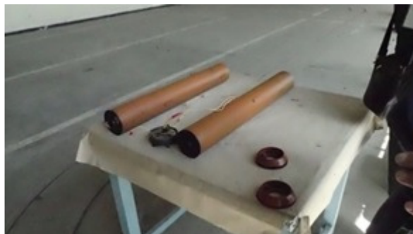
Fig. 6. Double base propellant fuel grains.
