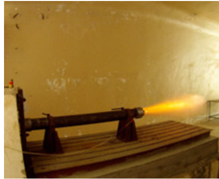
Fig. 8. Double base SRM during test firing.
