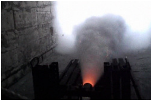
Fig. 7. Composite SRM during firing test.
