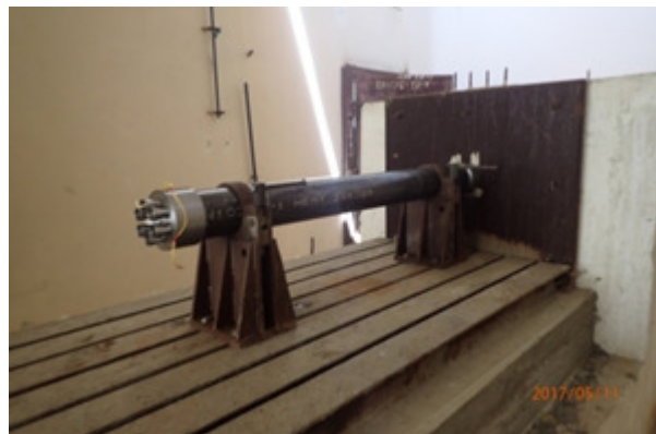
Fig. 4. Double base propellant SRM.
