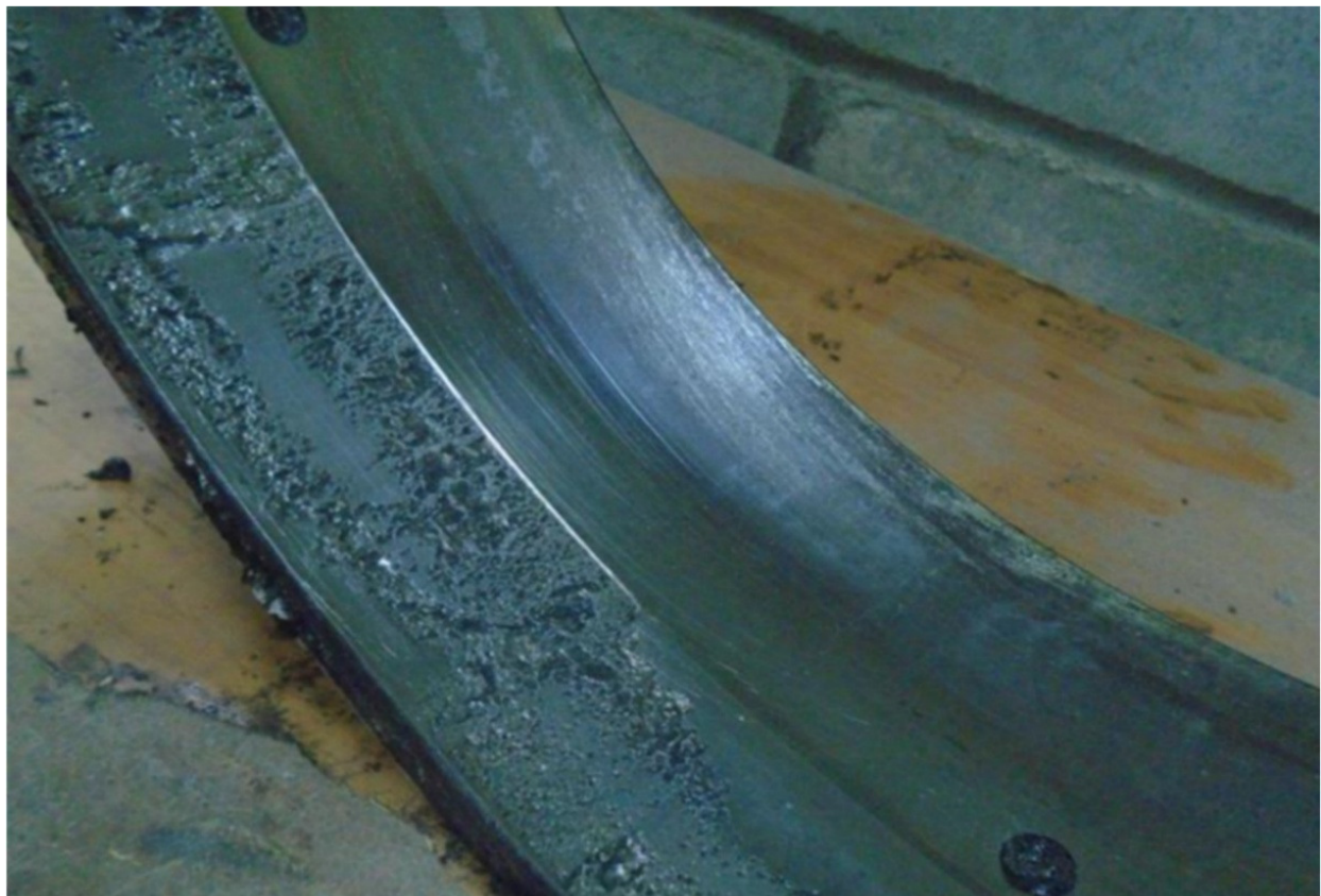
Fig. 15. Forming roll Drive Side bearing Outer Race Excessive Wear.
