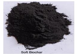
Figure (1). Picture of the Soft Corncob biochar used in the present study
