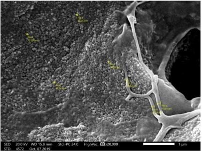
Plate (1). SEM micrograph of Soft corncob biochar
