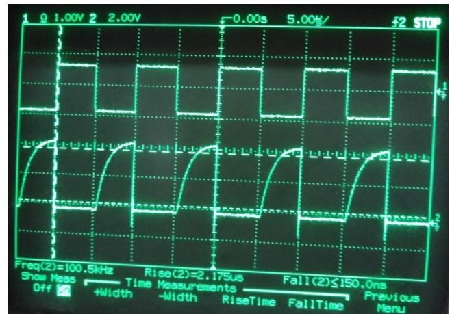
Fig. (15): Sample of measured output pulse (down) with reference input pulse (up) using a digital oscilloscope second group device two after 0.5 Gy gamma irradiation.
