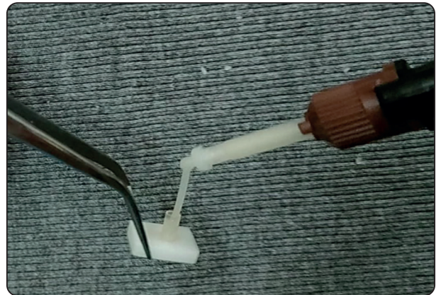
Fig. (2) Delivering the resin cement inside the silicone die using an "intra-canal" resin cement extension
