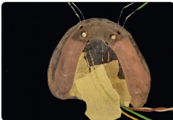
Fig. (7) Strain gauge fixation
