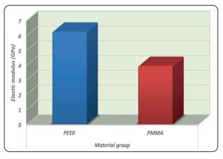
Fig. (2) Column chart comparing the mean scores Elastic Modulus of each group.
