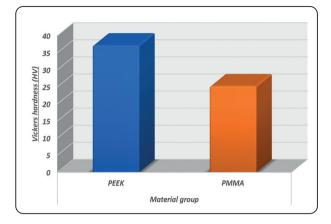
Fig (1) Column chart comparing the mean scores Vickers hardness of each group.
