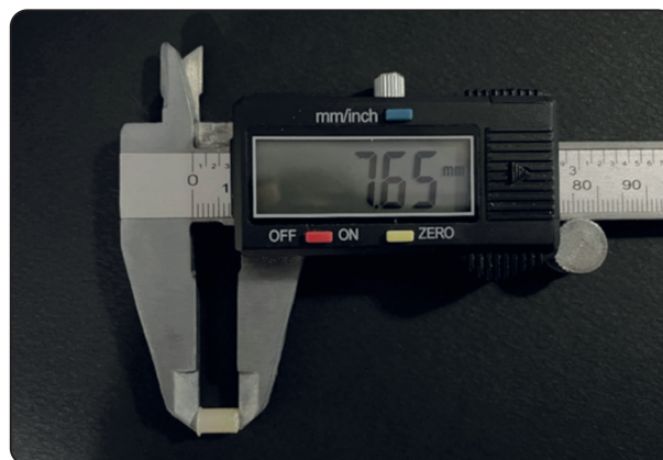
Fig. (1) Measuring the length of the specimen with the digital caliper for depth of cure test.
