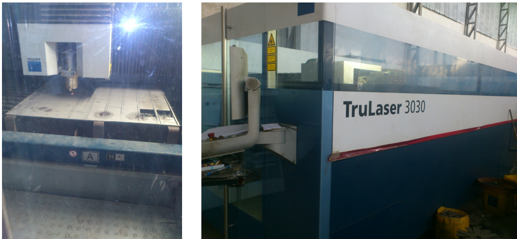
Fig. 1. The Laser Machine type (TruLaser 3030) used in cutting plates and test specimens.
