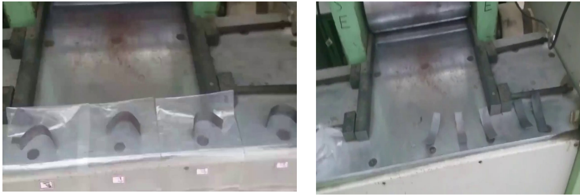
a. The samples shown after bending at certain pre-strain 3.1%.
