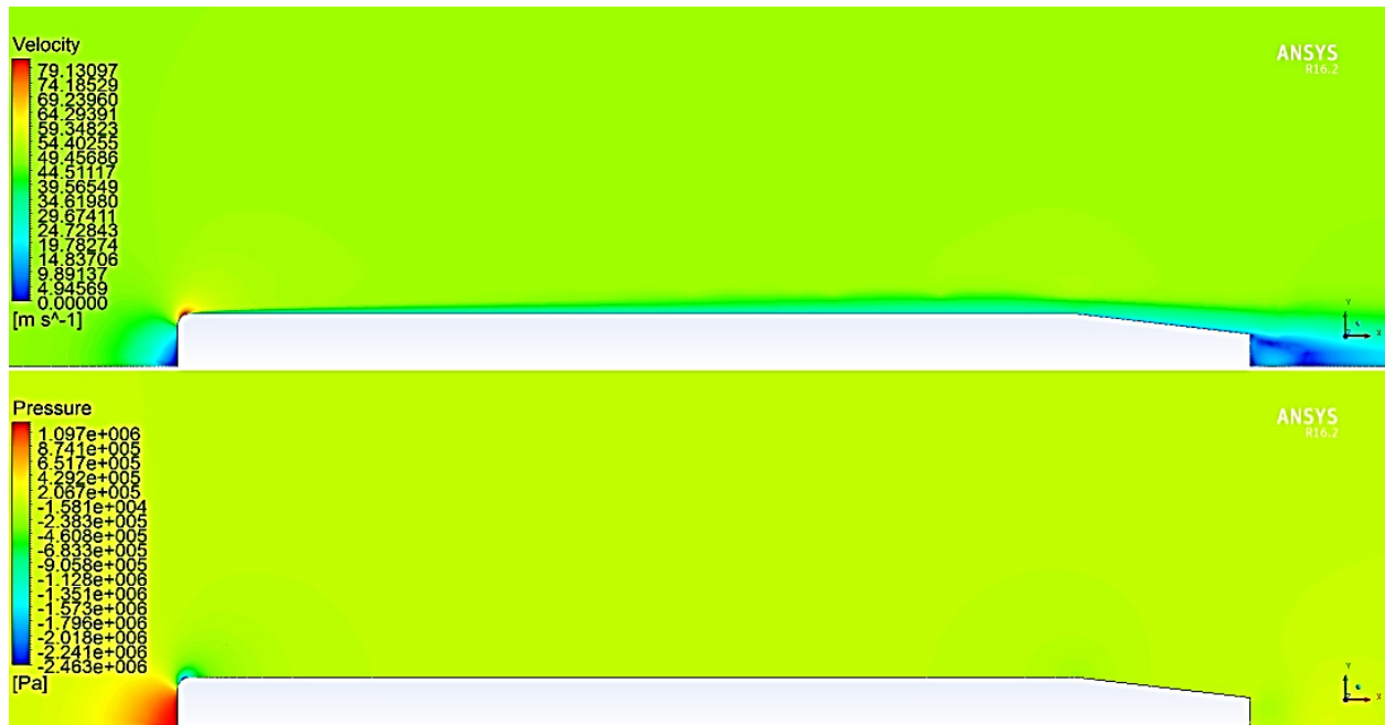
Fig. 14. Contours of velocity and pressure of stubbed nose profile, model (4), at velocity of 50 m/s.
