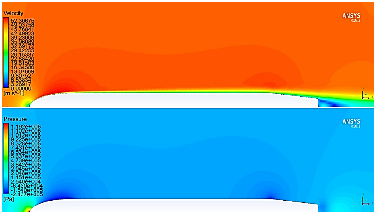
Fig. 15. Contours of velocity and pressure of elliptical nose profile, model (5), at velocity of 50 m/s.
