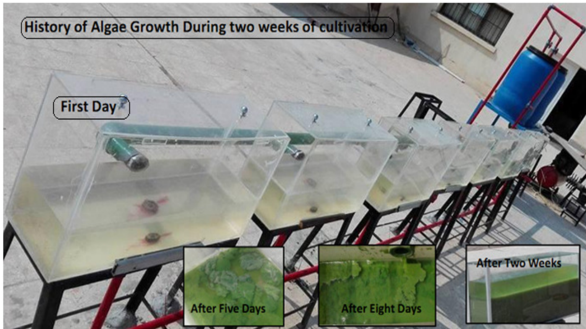
Fig. 3. Photos of the algae growth hestroy during one of the tested cultivation cycle.
