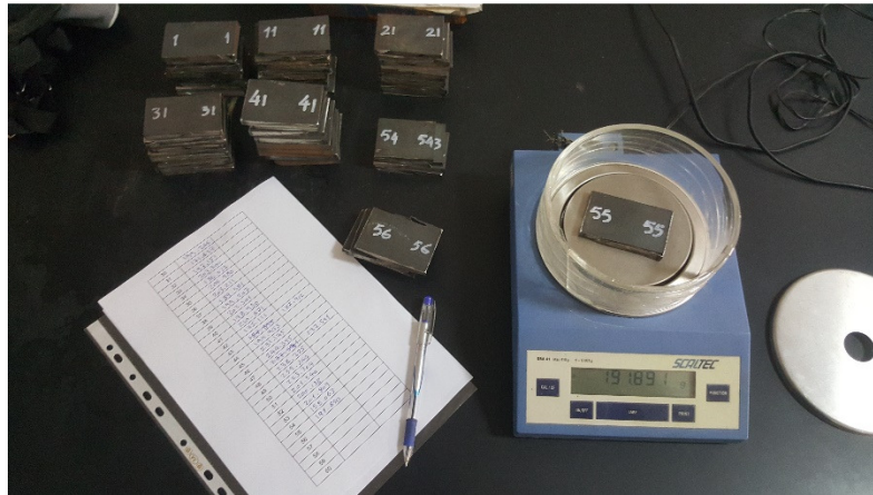
Fig. 3. Measuring weights of specimens in laboratory using SBA 41 sensitive scale.
