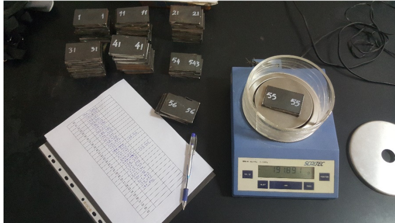
Fig. 1. Measuring weights of specimens in laboratory using SBA 41 sensitive scale.
