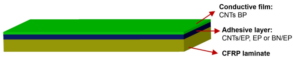
Fig. 3. Schematic of CFRP laminates with LSP system [4].
