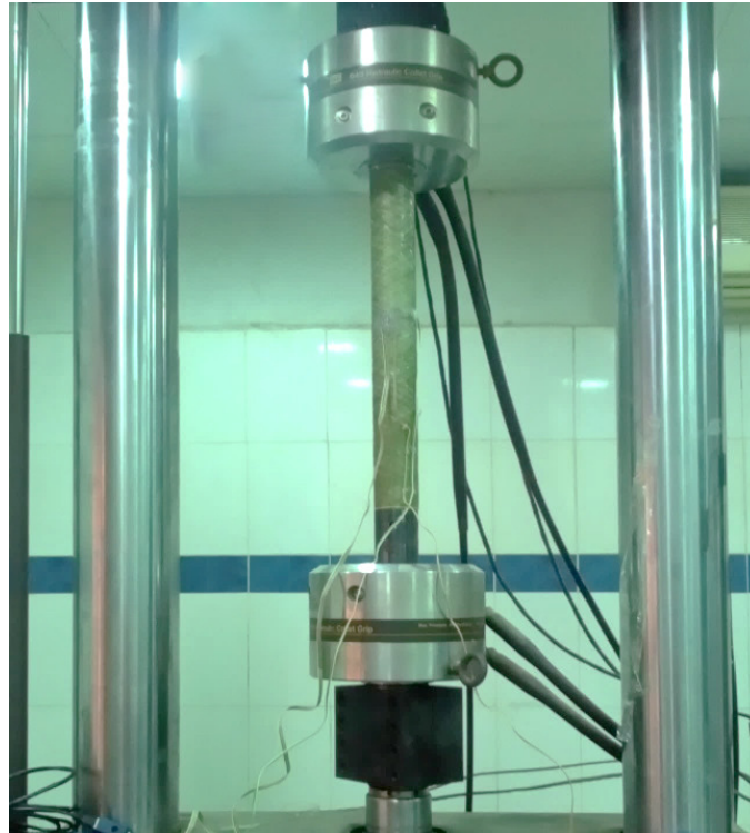
Fig.10. Axial compression test using MTS machine.
