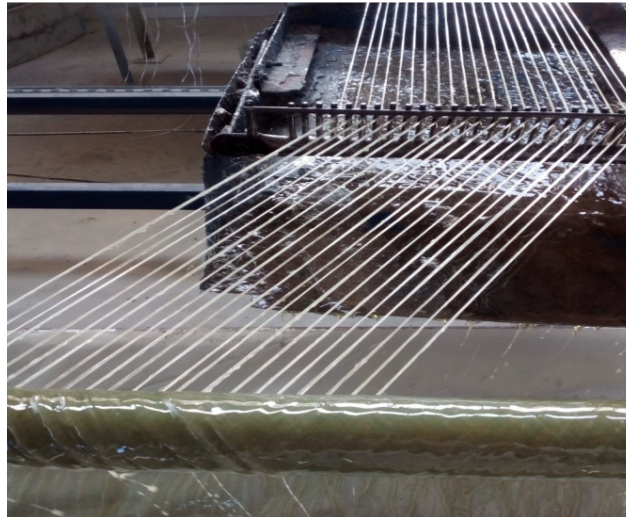
Fig. 1. Manufacturing of the composite tube by filament winding machine.
