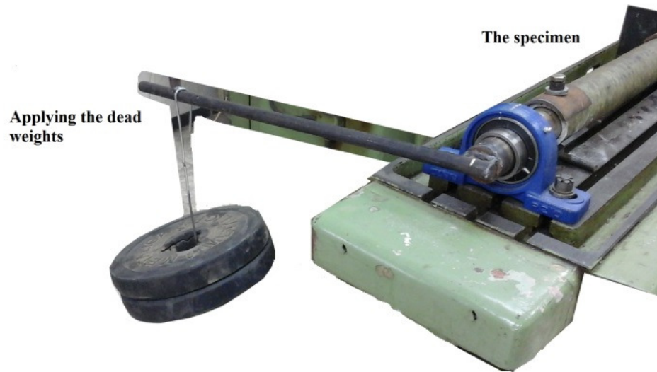
Fig. 7. Applying the dead weights to generate the required torques.
