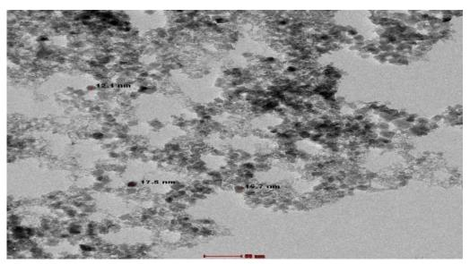
Fig. 3.TEM imaging of the prepared Fe<sub>2</sub>O<sub>3</sub> nanoparticles.
