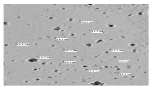
Fig. 4. TEM imaging of the prepared ZnO nanoparticles.
