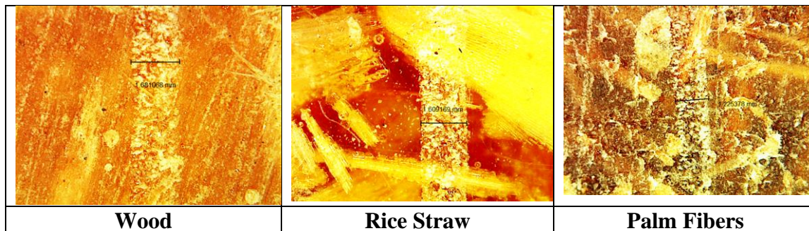
Fig. 6 The evidence of the scratch track on the tested composites.
