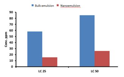
Fig. 4: LC<sub>25</sub>, LC<sub>50</sub> of nanoemulsion and bulk emulsion of *Cirtus sinensis* EO against 3<sup>rd</sup> instar *Culex pipiens* larvae after 24 hrs.
