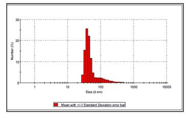
Fig. 1: Droplet size distribution of the nanoemulsion droplets by DLS.
