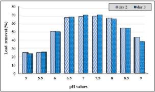
Fig. 7. Effect of initial medium pH on the bioremoval of lead by *B. amyloliquefaciens* MPA
