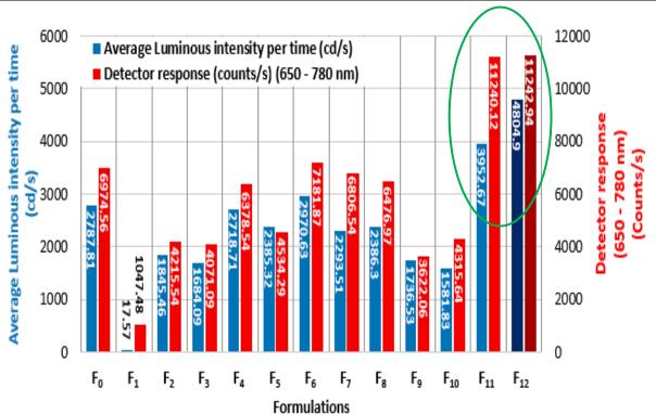
Fig. 11: Variation of average luminous intensity per time and detector response with different formulations
