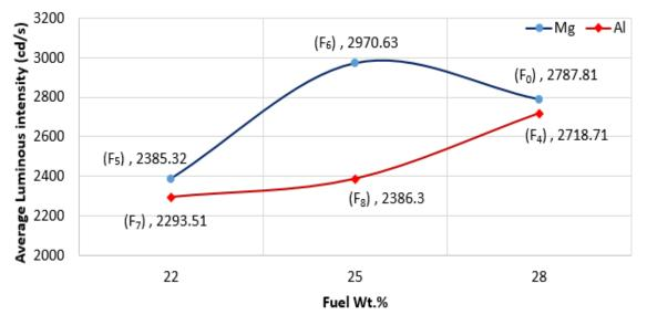
Fig. 6: Effect of fuel type/content on the luminous intensity in (cd/s)
