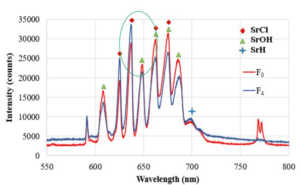
Fig. 5: The impact of fuel type on the imprint spectrum red flares
