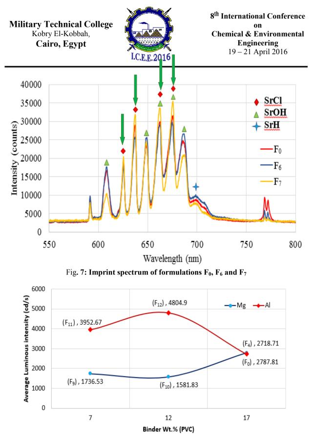
Fig. 8: Effect of color source to color intensifier on the luminous intensity in (cd/s)
