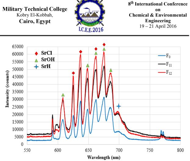
Fig. 9: Imprint spectra of developed red flared (F<sub>11</sub> and F<sub>12</sub>) to reference red flare (F<sub>0</sub>)
