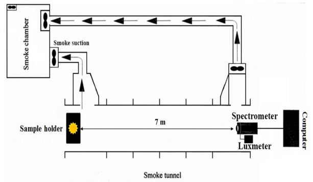
Fig. 2: Schematic for spectra measurements of developed red flares
