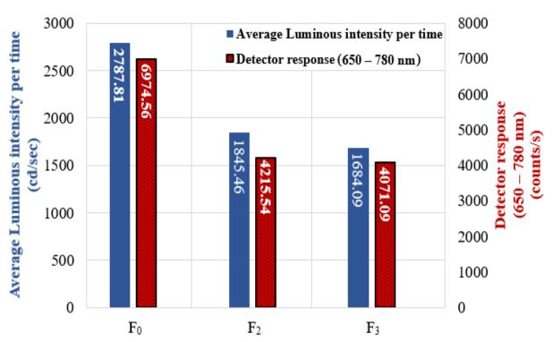
**Formulations** Fig. 3: Effect of binder type on the luminous intensity in (cd/s)
