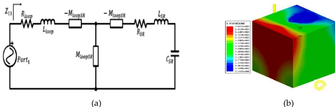
Figure 5. The CSLS Unit Cell: (a) Equivalent Circuit; (b) E-Field [V/m].
