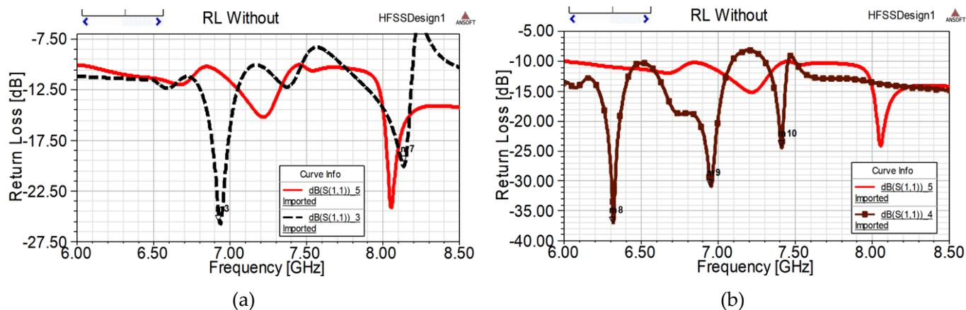
Figure 15. Horn Comparison Results: (a) Without and With 7-Elements Array ; (b) Without and With Triangular Array
