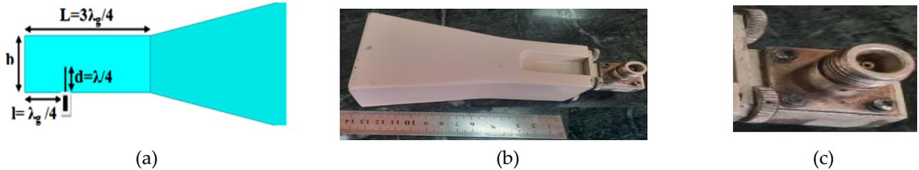
Figure 2. Horn With Waveguide Feeding Connection: (a) Design Dimensions;(b) Fabricated; (c) Connector
