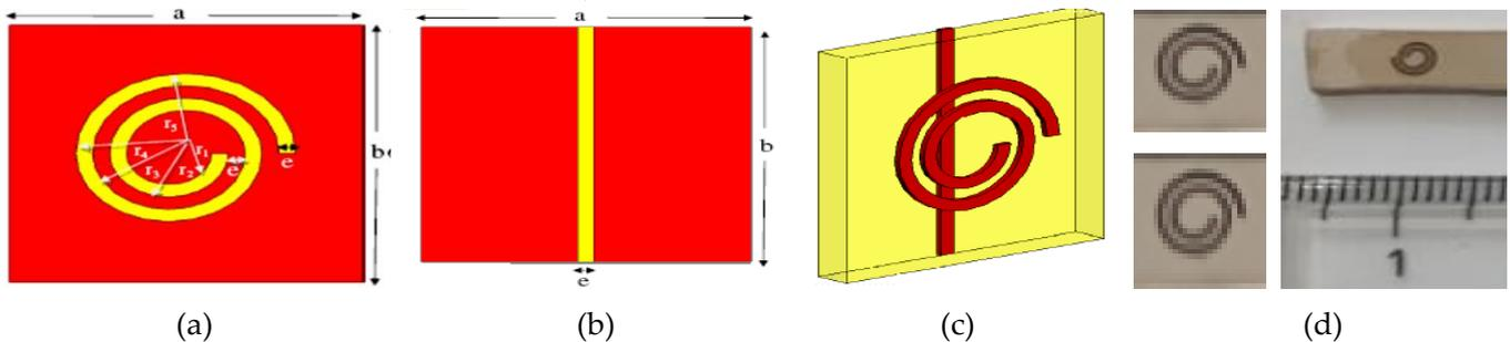
Figure 4. The CSLS Unit Cell Dimensions and Fabrication: (a) Front View; (b) Back View; (c) 3-D View; (d) Fabricated View;
