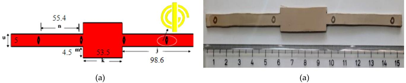
Figure 6. The CSLS Linear Array (a) Dimension [mm]; (b) Fabrication.
