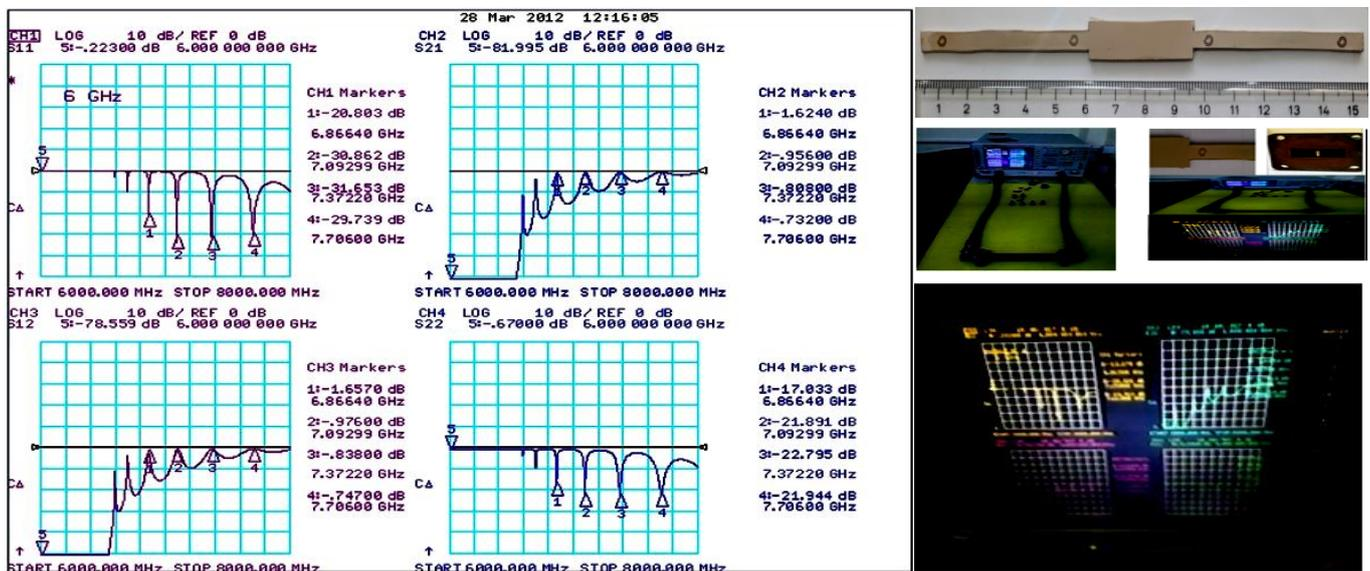
Figure 13. The Measured Results of CSLS linear Array Loaded in WR90 Rectangular Waveguide
