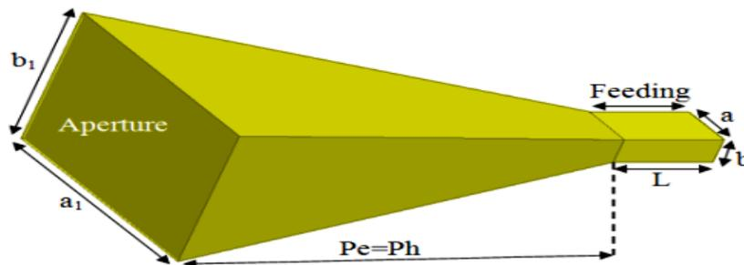
**Figure 1.** Pyramidal Horn Antenna Without CSLS Dimensions
