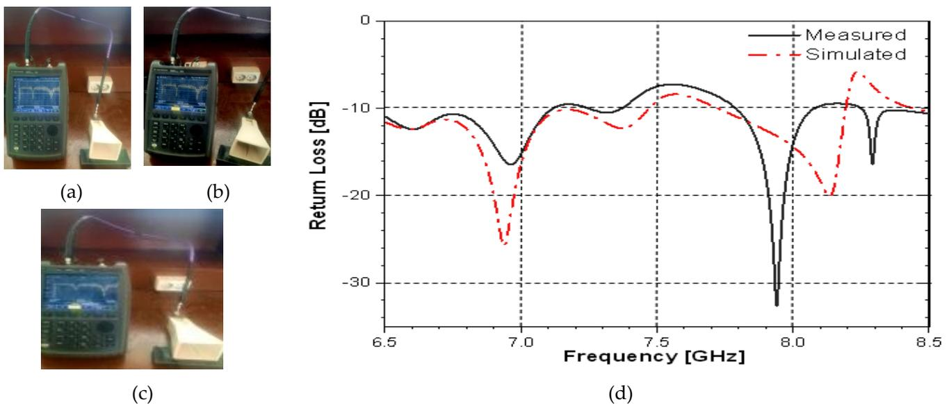
**Figure 14.** Laboratory Measurements and Comparison: (a) Horn Without CSLS Array; (b) Horn With CSLS Linear Array; (c) Horn With CSLS Triangular Array; (d) Comparison Between Simulation and Implementation Results.
