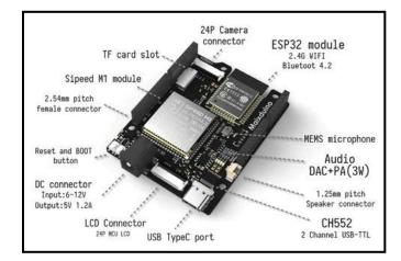
Figure 3: Sipeed Maixduino Kit RISC-V.
