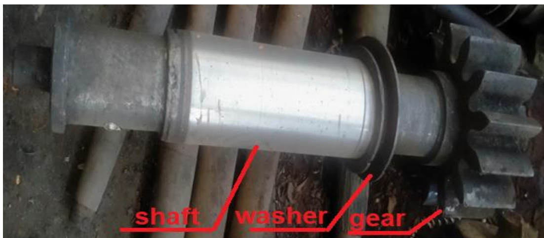
Figure 4. The shaft after lathing (Deshna factory).
