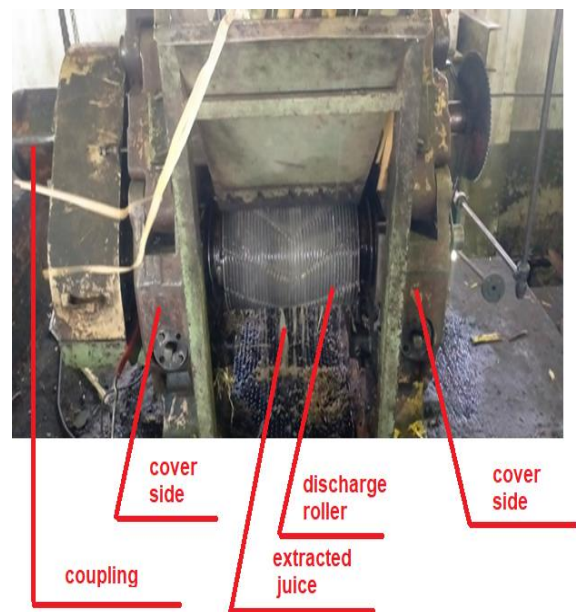
Figure 18. The juice path in unmodified mills is in the V-grooves only (Deshna factory).
