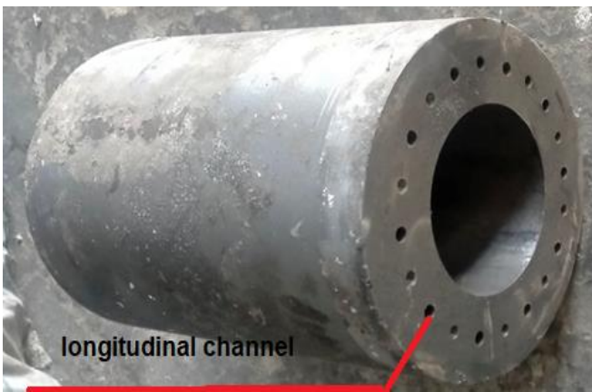
Figure 6. The shell after drilling the longitudinal channels (Deshna factory).
