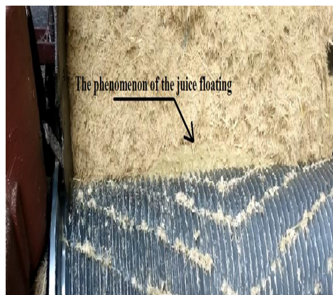
Figure 12. The phenomenon of flotation in the primary mill of the Dishna factories.
