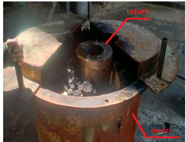
Figure 7. The shell inside the oven before the fitting process (Deshna factory).
