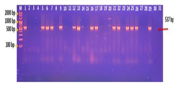
Fig. 2. Agarose gel electrophoresis shows conventional PCR analysis of 16S rRNA gene in PCR products of cattle blood samples to detect S bovis.
