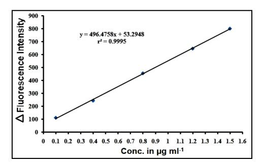
Figure (8): Calibration Graph of ADV with Eosin – Y at  $\lambda_{em}$  544 nm.
