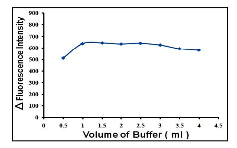
Figure (5): Effect of Buffer Volume on the fluorescence of ADV (1.2 μg ml<sup>-1</sup>) Reaction Product with Eosin - Y at λem 544 nm.
