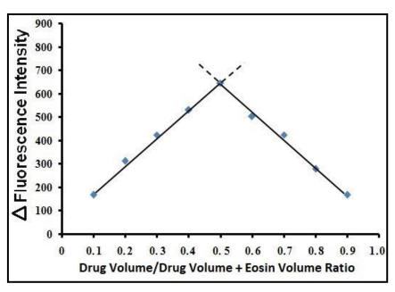
Figure (7): Stoichiometry of The Reaction of of ADV (4.39 x  $10^{-6}$  M) With Eosin –Y (4.39 x  $10^{-6}$  M) by Continuous Variation (Job's) Method at  $\lambda$  em 544 nm.
