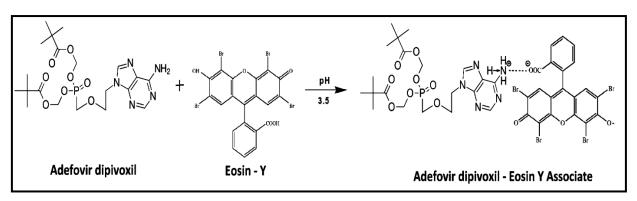
Fig 9. The supposed reaction pathway between ADV and Eosin - Y
