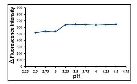
Figure (4): Effect of pH on The Fluorescence of ADV (1.2  $\mu$ g ml<sup>-1</sup>) Reaction Product with Eosin - Y at  $\lambda$ em 544 nm.
