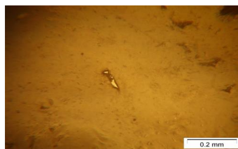
Fig.8. Apatite present as fine disseminated grains within the hematite matrix [24]
