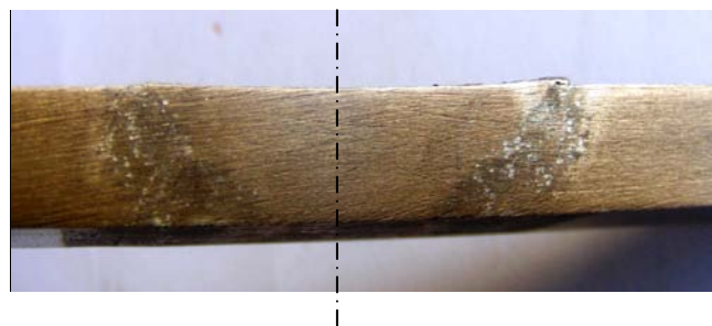
Figure. 11 Optical macrograph of the transverse welding plane after 100 hrs immersion in the 3.5% NaCl solution.
