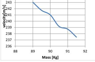
**Fig. 12**. Maximum velocity versus mass variation with constant ( $x_{cq}$ ,  $\theta_0$ ,  $v_0$ ).
