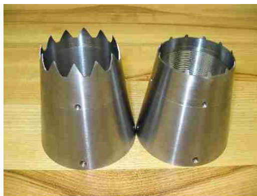
Fig. 6. Nozzle tabs (right) and chevron (left).
