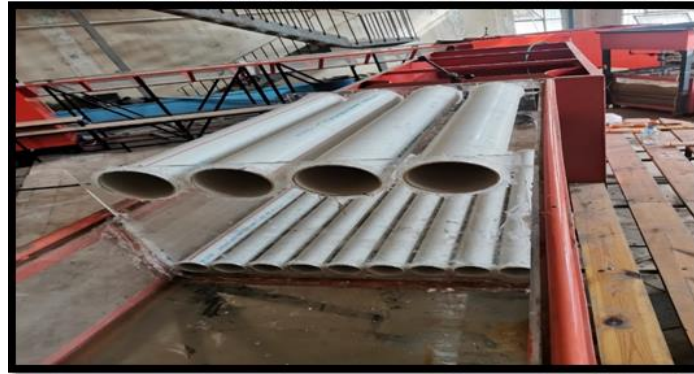
Figure (4) Installing the model in the flume
