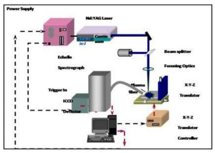
Fig. (4): LIBS experimental setup.
