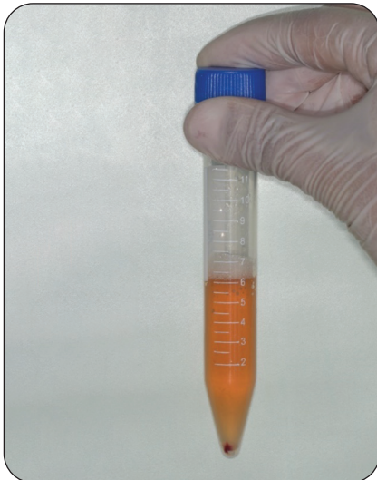
Fig. (4) Cell isolate was then washed using balanced salt solution and centrifuged at 2000 rpm for 10 min
