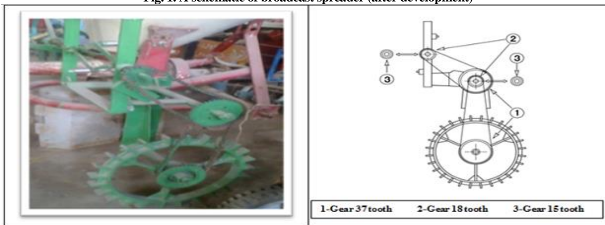
Fig. 2. Developed transmission device of spreader
