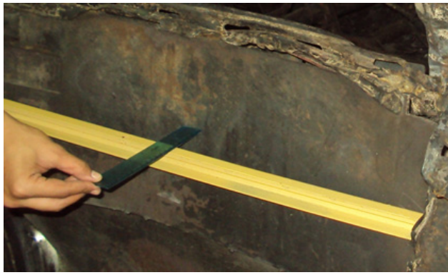
Fig. 3: Effect of 150 kg of TNT at a distance of 3m on 7mm ArmoX-500 plate.
