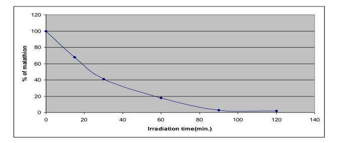
Fig.7. Effect of variation of irradiation time on the photodecontamination process of malathion
