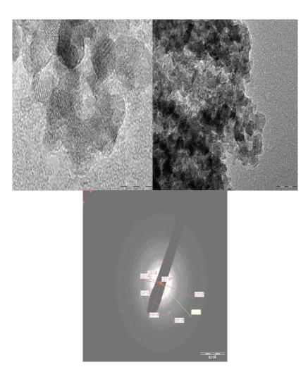
Fig.3. TEM and HEED images of TiO<sub>2</sub> nano particles synthesized
