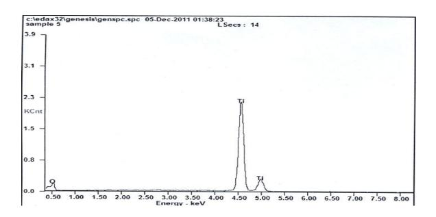
Fig.2. EDX spectrum of TiO<sub>2</sub> nano particles
