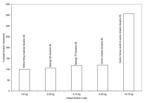
Fig. 13. Impact broken resistance (locations-B).
