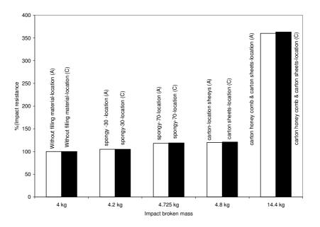
Fig. 12. Impact broken resistance (locations-A & C).
