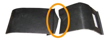
Fig. 11. Broken specimen (tested with filling material double layer of carton as a honey comb)
