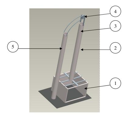
1- base box 2- hollow shaft 3-drop weight with wire 4- pulley 5-fixed arm.
