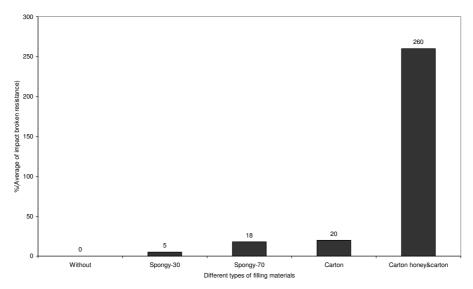
Fig. 14. Average impact broken resistance of bumper.
