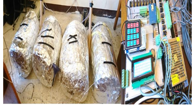
Fig. 1. Three tanks insulated using krino material and the fourth tank insulated by glass wool
