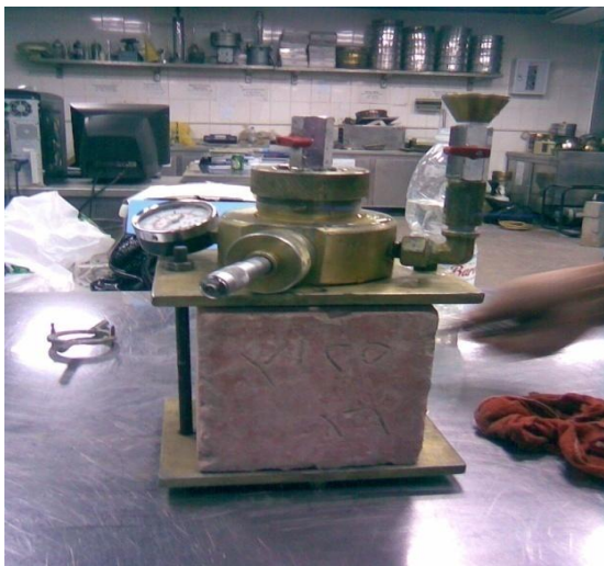
Fig (2) permeability test for hardened concrete
