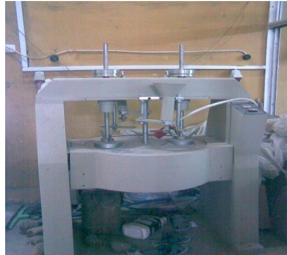
Fig (3) Abrasion test for hardened concrete
