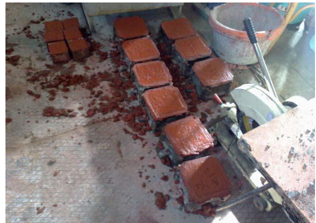
Fig (1) Red concrete specimens in the slandered forms after casting
