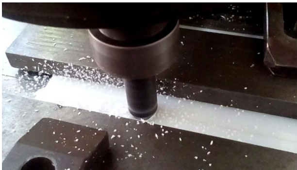
Fig. 12: High rotation speed caused ejection of polymer
