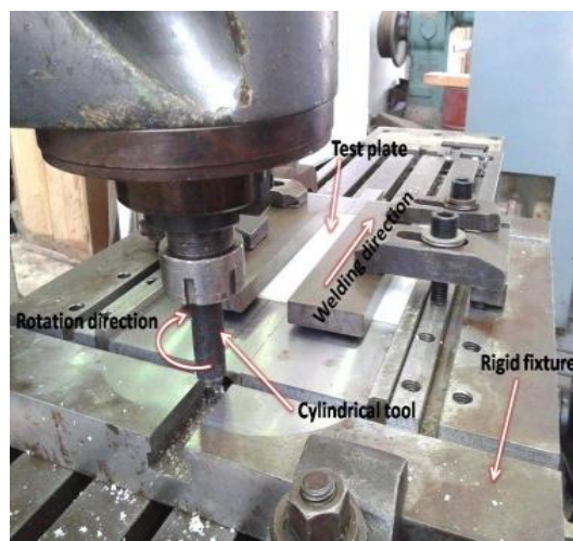
Fig. 3: Friction stir welding operation
