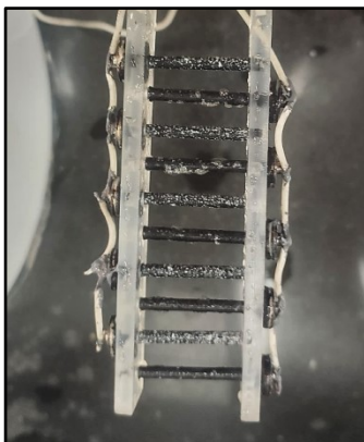
Fig. 3 The dissolved solids in the water accumulated on the electrodes after the electrolysis process
