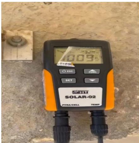
FIGURE 4. SOLAR-02 environmental parameters data logger.
