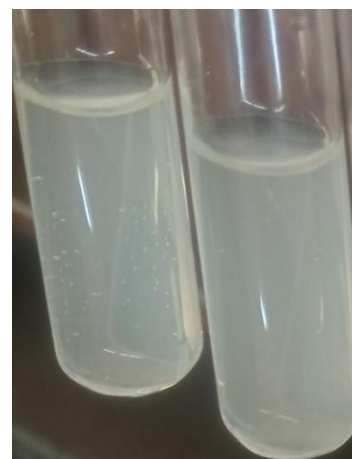
Figure 7. The observed turbidity between Cr(VI) and ethanol at [Cr(VI)] = 88 Ppm, and EtOH% = 30 %.
