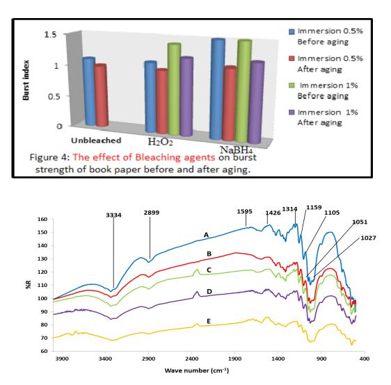
Fig. 4a. FT-IR spectroscopy of cotton linter paper before aging: (A) unbleached, (B) 0.5 % H<sub>2</sub>O<sub>2</sub>, (C) 1% H<sub>2</sub>O<sub>2</sub>, (D) 0.5 % NaBH<sub>4</sub>, and (E) 1% NaBH<sub>4</sub>.
