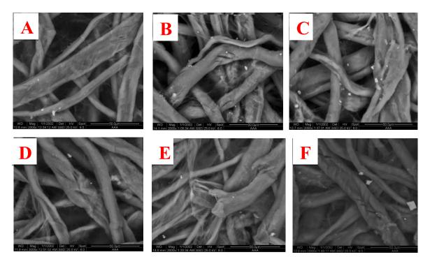
Fig. 5. SEM of non aged cotton linter paper ((A) unbleached, (B) bleached by H<sub>2</sub>O<sub>2</sub>, (C) bleached by NaBH<sub>4</sub>); aged cotton linter paper ((E) bleached by H<sub>2</sub>O<sub>2</sub>, (F) bleached by NaBH<sub>4</sub>)
