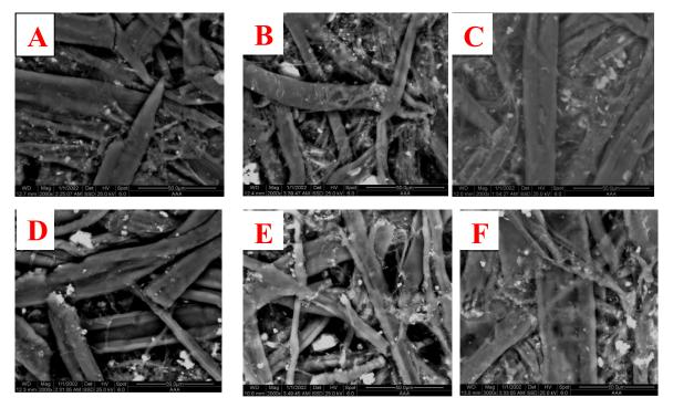
Fig. 6. SEM of non aged book paper ((A) unbleached, (B) bleached by H<sub>2</sub>O<sub>2</sub>, (C) bleached by NaBH<sub>4</sub>); aged book paper ((E) bleached by H<sub>2</sub>O<sub>2</sub>, (F) bleached by NaBH<sub>4</sub>).
