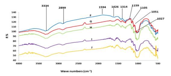
Fig. 4b. FT-IR spectroscopy of cotton linter paper after aging: (F) unbleached, (G) 0.5 % H<sub>2</sub>O<sub>2</sub>, (H) 1% H<sub>2</sub>O<sub>2</sub>,(I) 0.5 % NaBH<sub>4</sub>, and (J) 1% NaBH<sub>4</sub>.
