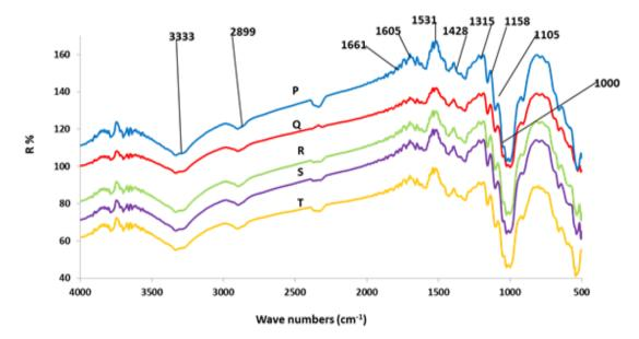
Fig. 4d. FT-IR spectroscopy of book paper after aging: (P) unbleached, (Q) 0.5 % H<sub>2</sub>O<sub>2</sub>, (R) 1% H<sub>2</sub>O<sub>2</sub>, (S) 0.5 % NaBH<sub>4</sub> and (T) 1% NaBH<sub>4</sub>.
