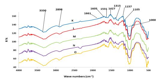
Fig. 4c. FT-IR spectroscopy of book paper before aging: (K) unbleached, (L) 0.5 % H<sub>2</sub>O<sub>2</sub>, (M) 1% H<sub>2</sub>O<sub>2</sub>, (N) 0.5 % NaBH<sub>4</sub> and (O) 1% NaBH<sub>4</sub>.
