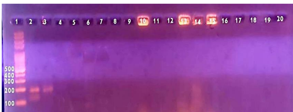
Photo 2: Agarose gel electrophoresis for HSV DNA polymerase gene amplicons in conjunctival swabs Lane 1 represents 100-bp DNA molecular size marker, lane 2,3 are positive samples for the gene (179 bp)
